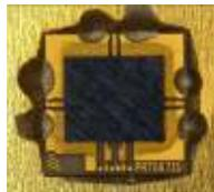
**Note:** \* Epoxy was used to connect top metal GND to bottom GND plane for improved RF probe to substrate transition.
