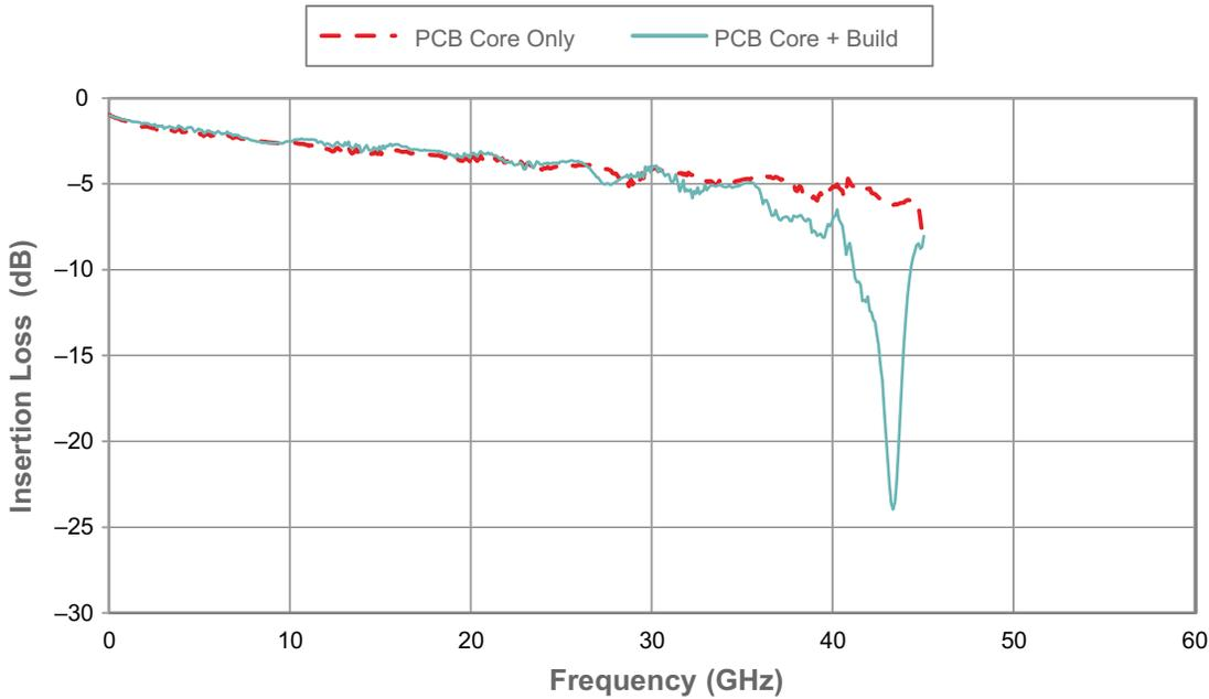
**Note:** \* PCB core only: PRT61038 substrate carrier with RF connectors; PCB core + build: 8 mil Rogers 4003 plus 370HR laminate (62 mil total) with RF connectors.
