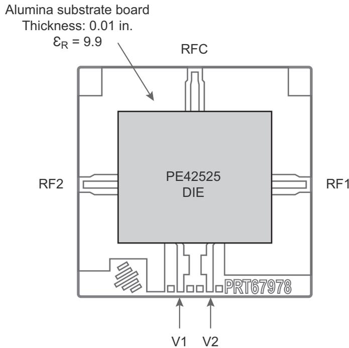
To minimize unwanted wicking of individual solder balls from the local connection point, use a solder stop such as a marking, protective polymer layer, or other material recommended by the substrate manufacturer. The solder stop thickness should be 15–25  $\mu\text{m}$  to prevent the solder wicking from touching the face of the PE42525 die.
