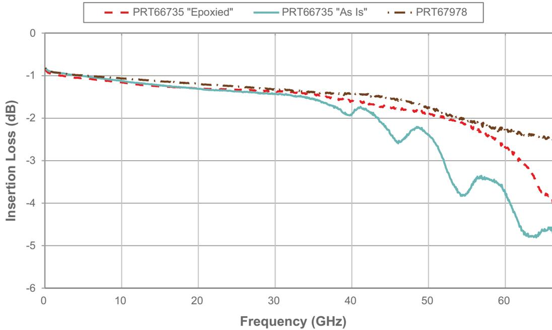
**Note:** \* Comparison is between 10 mil alumina substrate carriers PRT66735 (with and without epoxy) and PRT67978 metalization and via patterns. PRT67978 is the recommended pattern. PRT66735 with epoxy grounding was used for characterization.
