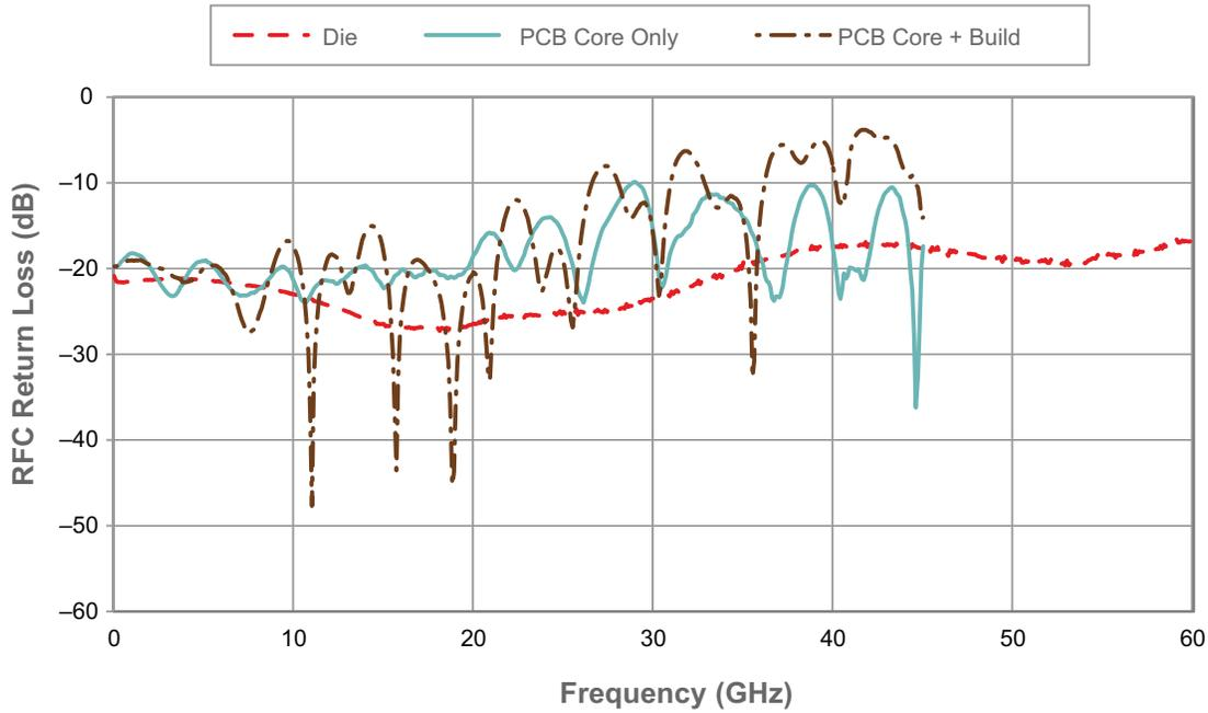
Note: \* Die: RF probe on PRT67978 alumina carrier; PCB core only: PRT61038 substrate carrier with RF connectors; PCB core + build: 8 mil Rogers 4003 plus 370HR laminate (62 mil total) with RF connectors.
