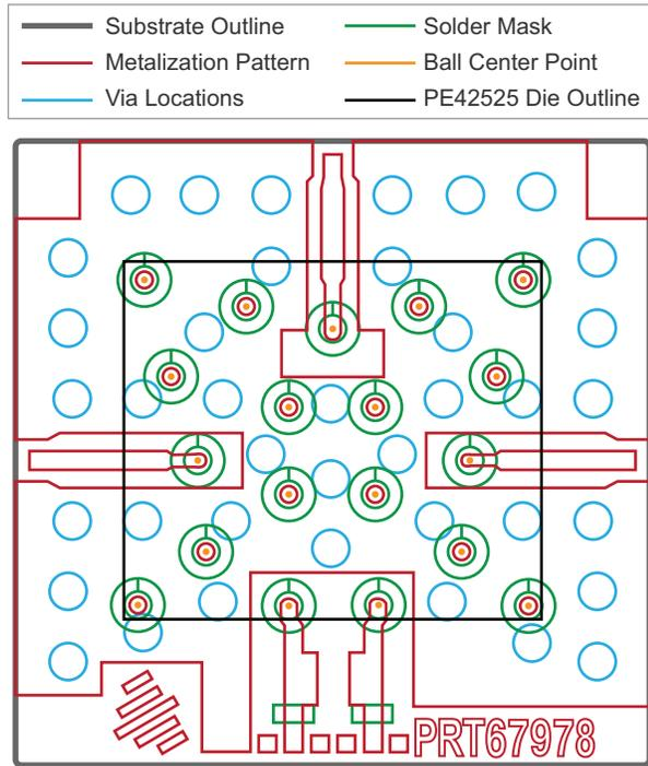
RF performance can be affected by metalzation and via patterns. **Figure 4**, for example, shows changes in insertion loss levels due to grounding differences near the RF probe transitions for the PRT66735. For comparison, the substrate PRT67978 used for present sampling of the PE42525 and PE426525 is also shown. The epoxied PRT66735 substrate and edge-wrapped PRT67978 substrate eliminate insertion ripple for frequencies over 40 GHz.
