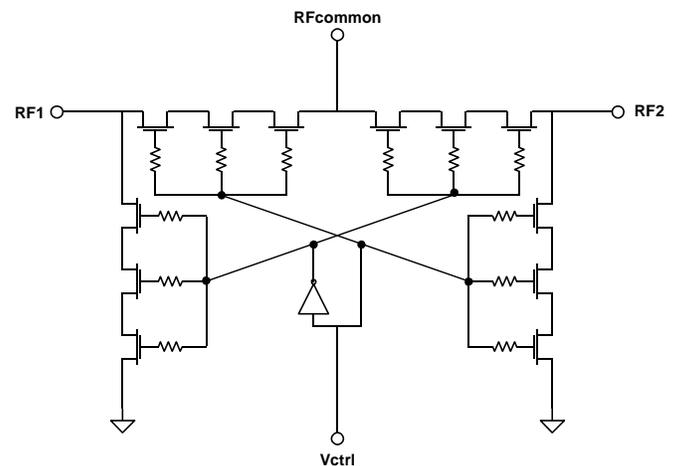
typically occurs when gate voltage is  $-2V$  to  $-3V$  so the gate is normally biased at  $0V$ .
