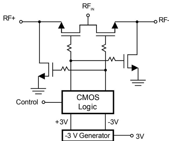
Figure 4 shows the block diagram of a high-power UltraCMOS RF switch, including integrated NVG and logic, providing true single-wire control.
