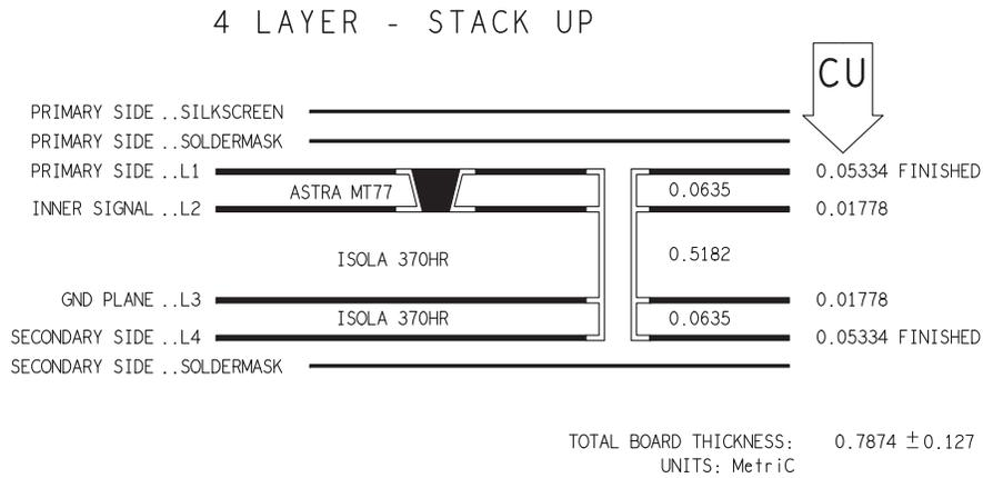
In general, for different RF core dielectrics and thicknesses, the critical dimensions of line width and spacing and via diameter can be readily scaled to accommodate the specific thickness requirements.
