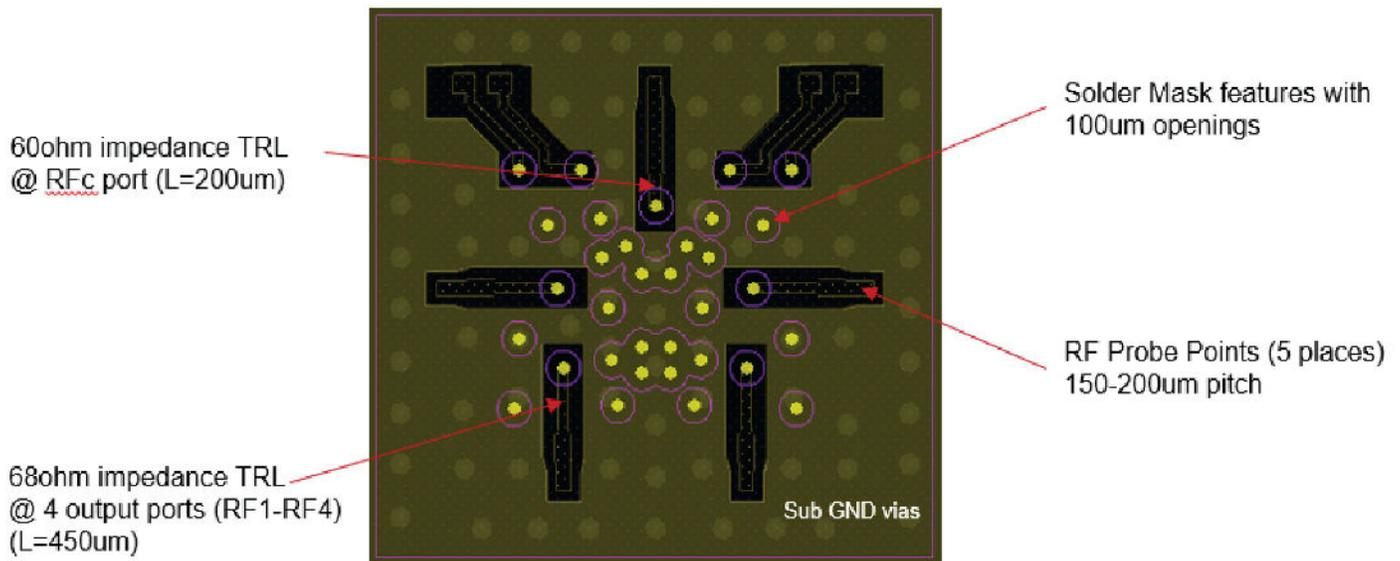
**Figure 3 ■ PRT-80235 Printed Circuit Board Composition**
